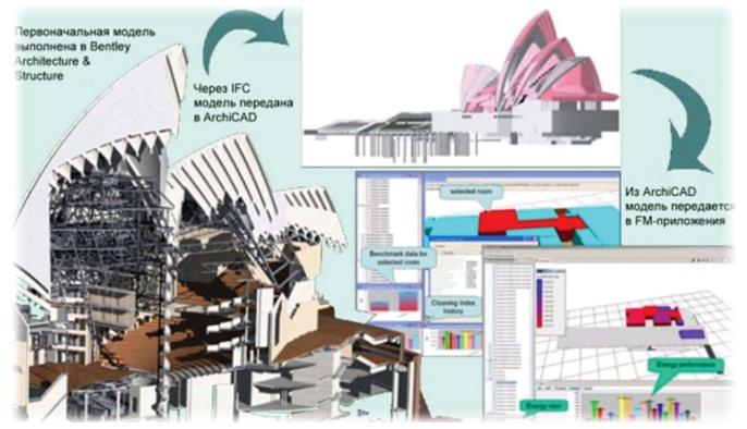
Figure 1: Diagram of data transfer of the building information model between the various programs involved in its creation using the IFC format
